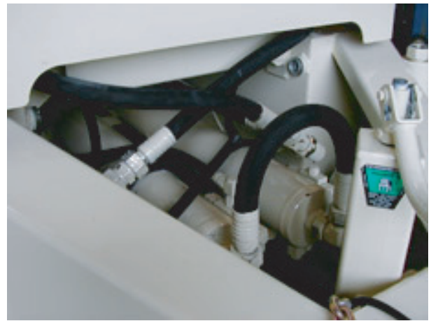
Figure 40 Hose configuration for rod side pumping with a SP 2000
