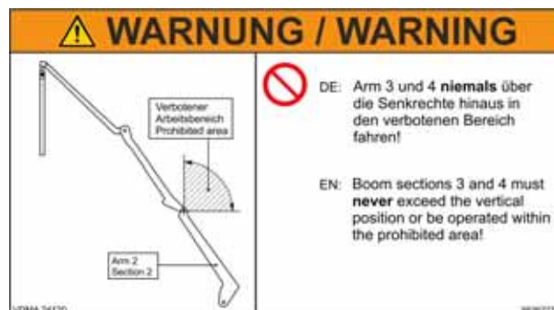
Fig. 250 Prohibited area for boom sections 3 and 4
