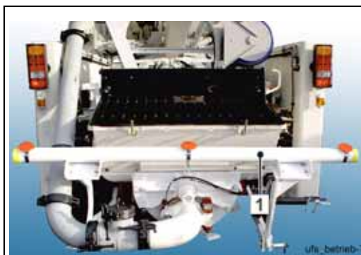
Fig. 263 Underride protection in operating position
