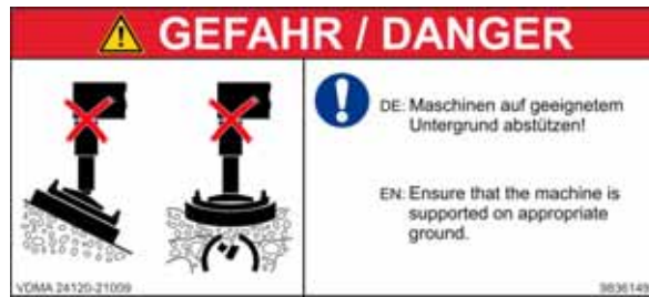
Fig. 128 Unsuitable set-up ground
