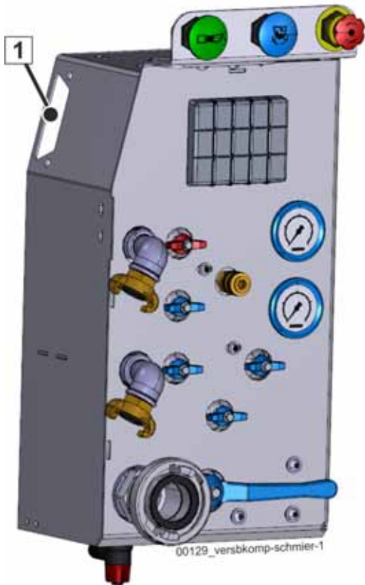
Fig. 310: Greasing strip on truck-mounted concrete pumps
