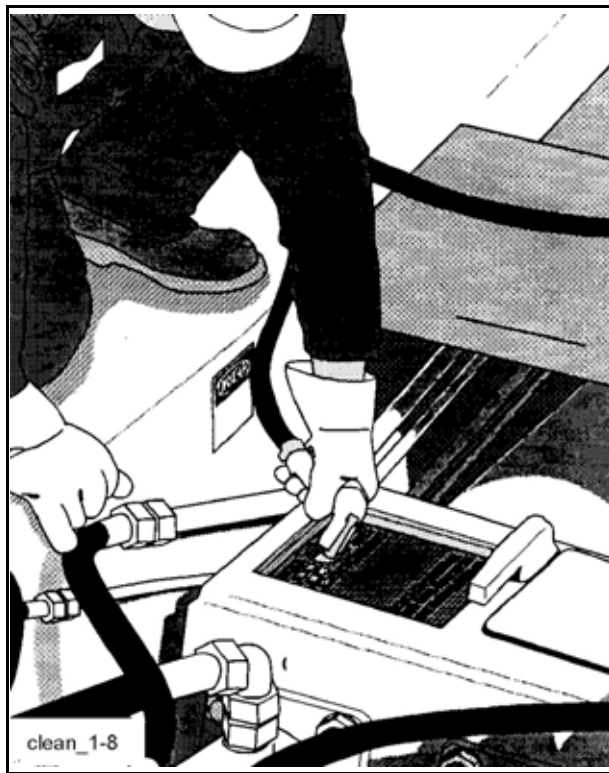
clean_1-8 Fig. 240 Hose out water box
