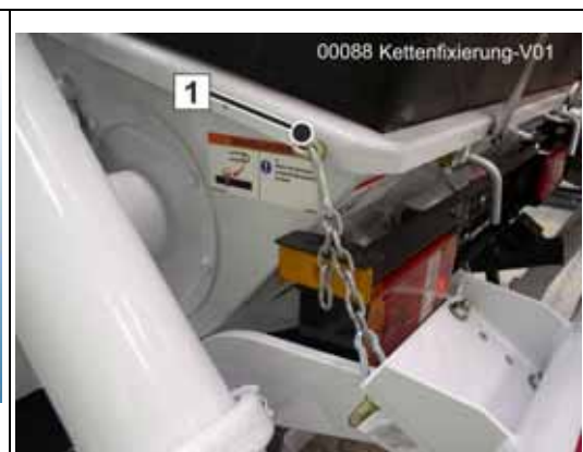
Fig. 264 Chain fastener for underride protection in operating position
