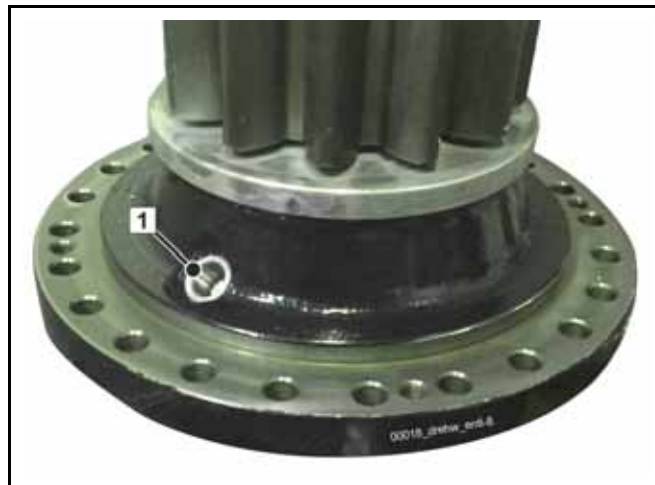
Fig. 301 Oil fill opening
