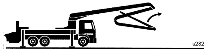
Fig. 194 Placing boom section 4
