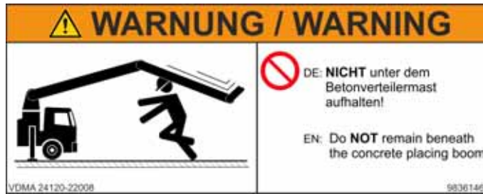
Fig. 168 Danger zone of placing boom
