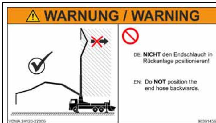
Fig. 2 Placing boom in backwards position
