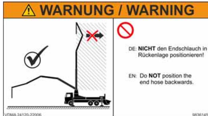
Fig. 166 Placing boom in backwards position
