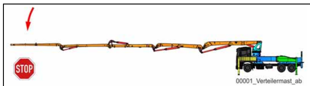
Fig. 169 Placing boom extended, movement stopped
