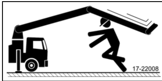
Fig. 4 Danger zone of placing boom
