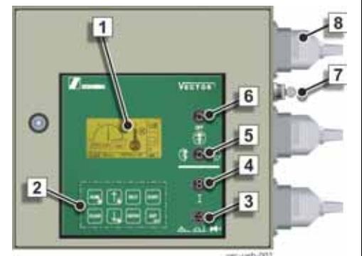
Fig. 72 Switch cabinet for VECTOR control
