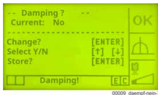
Fig. 653 Vibration damping disabled
