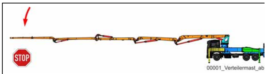
Fig. 167 Placing boom extended, movement stopped
