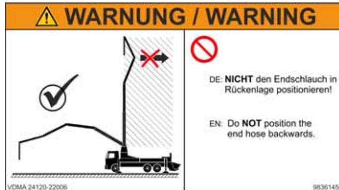
Fig. 164 Placing boom in backwards position
