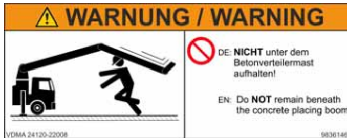
Fig. 166 Danger zone of placing boom
