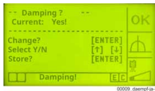
Fig. 81 Vibration damper ON
